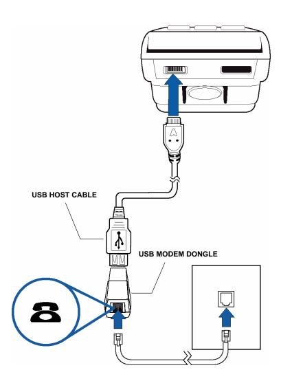
Figure 7 V<sup>x</sup>670 USB Modem Dongle Connection
